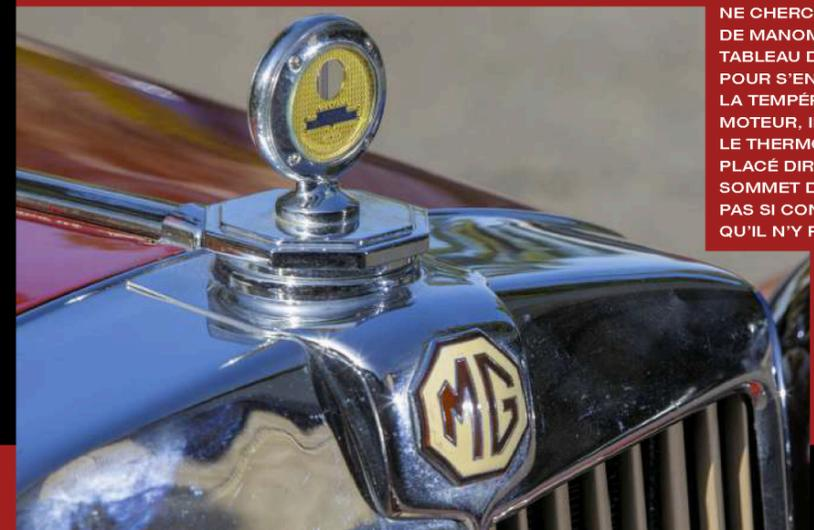
NE CHERCHEZ PAS DE MANOMÈTRE AU TABLEAU DE BORD. POUR S'ENQUÉRIR DE LA TEMPÉRATURE DU MOTEUR, IL FAUT SCRUTER LE THERMOMÈTRE PLACÉ DIRECTEMENT AU SOMMET DU RADIATEUR. PAS SI CONTRAIGNANT QU'IL N'Y PARAÎT.
